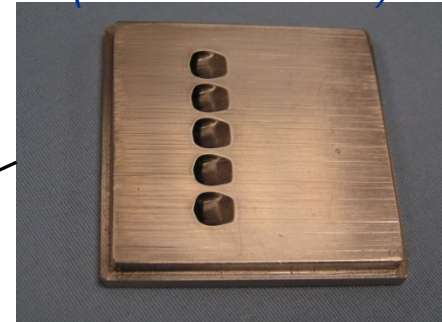
Flat Plate Test Specimen (50 x 50 x 6 mm)
